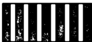
FIG. 3 Stroboscopic Lines Opening When Timer is Adjusted to Exactly 200 r/min
