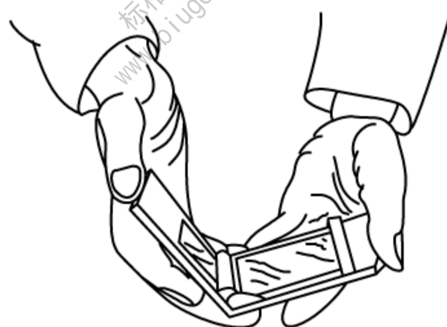
Figure 2 — Type 1 bend test apparatus in use
