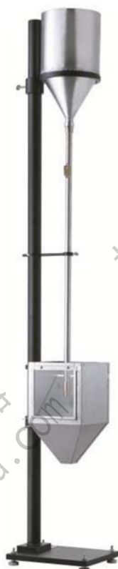
FIG. 1 Apparatus for Falling Sand Abrasion Test
