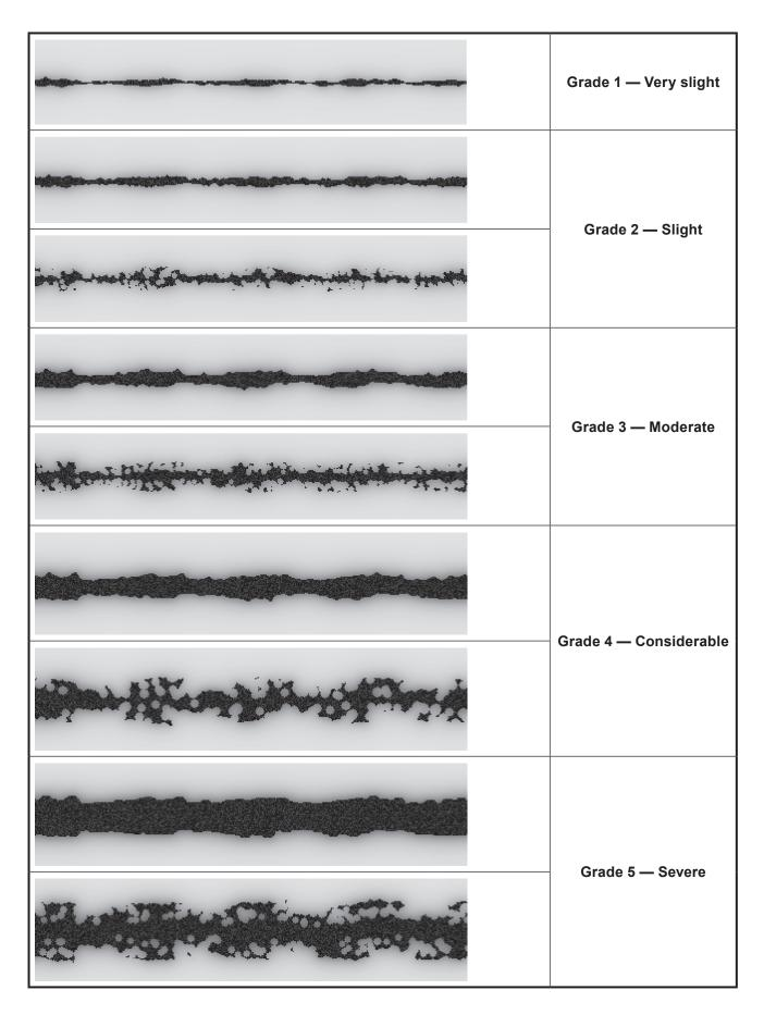
Figure 2 — Pictorial standards for assessment of delamination and corrosion around a scribe (approximate scale 1:1)
